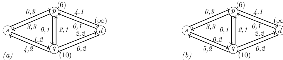
FIGURE 4. (a) The renovated network of the network in Figure 3(c) with respect to \gamma_p^3 . (b) The residual network after applying MCC Algorithm on the network in (a).
